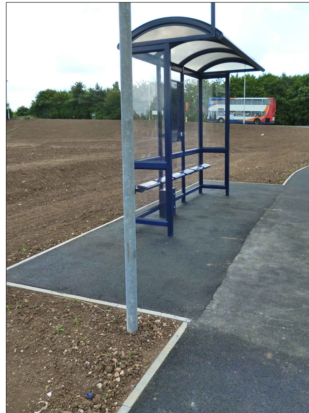
Example of a Queensbury 'Arun' bus shelter with barrel roof, incorporating seating, enclosed bus timetable board, electricity intake unit for real time passenger information capability and a bracket for bus flag. Note, the above example has half end panels rather than full end panels.
